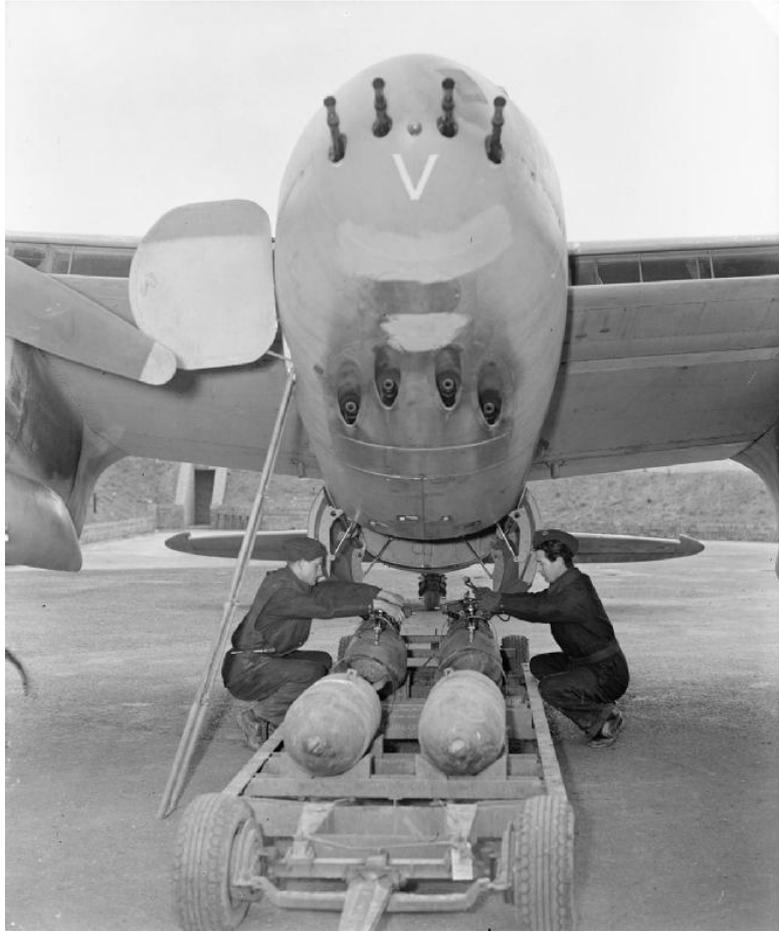
fig. 14: Armours load four 500 lbs MC bombs into the bomb-bay of a de Havilland DH.98 Mosquito fighter-bomber (FB) Mk VI, 1944. This type of aircraft was armed with four .303 in Browning machine guns and four 20 mm cannons.<sup>17</sup>
