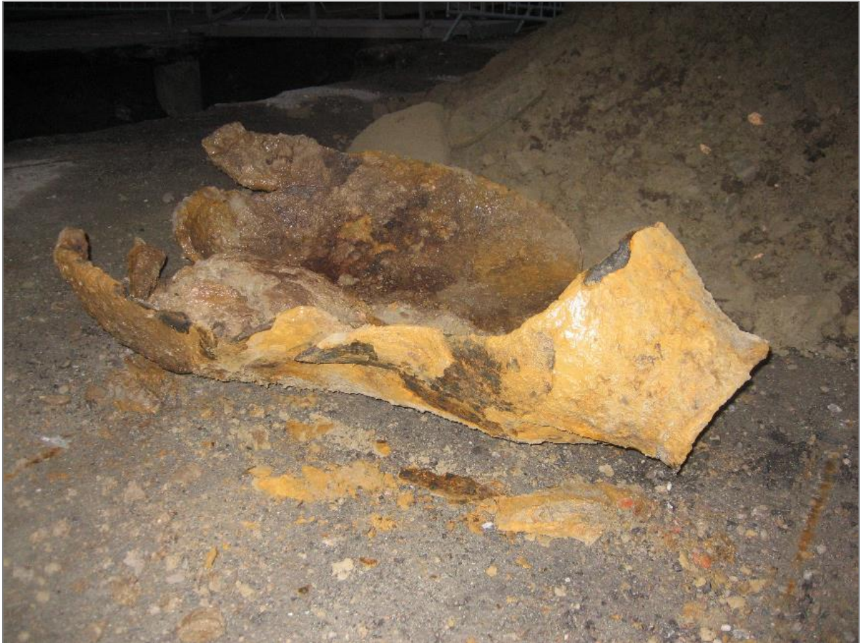
Figure 34: Photo of a detonated bomb recovered at Herøya. The bomb resembles a US M43 500lb bomb. 63
