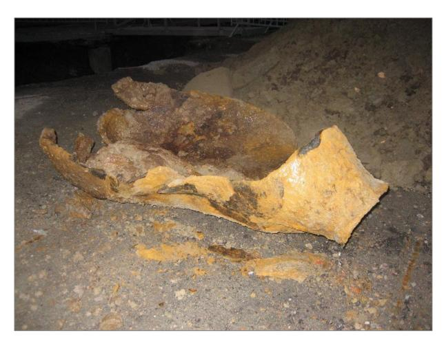
Figure 34: Photo of a detonated bomb recovered at Herøya. The bomb resembles a US M43  $\,$  500lb bomb.  $^{63}$
