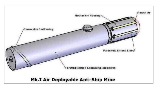
Figure 30: MK I Air-Deployable Anti-ship mine<sup>60</sup>
