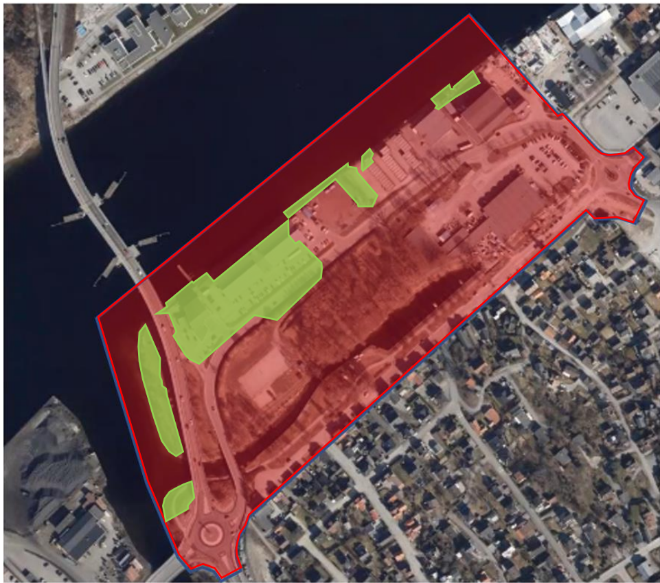
fig. 21: Above: Risk map for aerial bombs in the project area (red: very high risk; purple: very high risk under the backfill package). Below: Risk map for rockets in the project area (red: very high risk).
