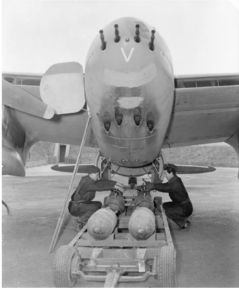
fig. 14: Armours load four 500 lbs MC bombs into the bomb-bay of a de Havilland DH.98 Mosquito fighter-bomber (FB) Mk VI, 1944. This type of aircraft was armed with four .303 in Browning machine guns and four 20 mm cannons. 17
